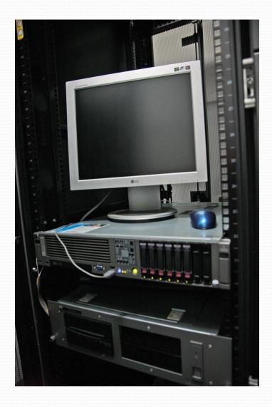
FTP/HTTP Server HP-DL380G5: RAM - 24 GB; HDD - 6x146GB 10K with a storage device HP StorageWorks 3U SDLT 600 Internal WW Tape Drive.
